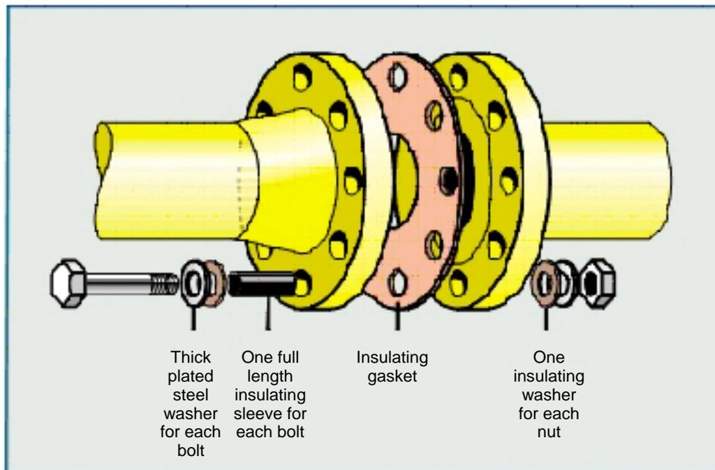
Figure 17.1 - Schematic diagram of insulating flange
