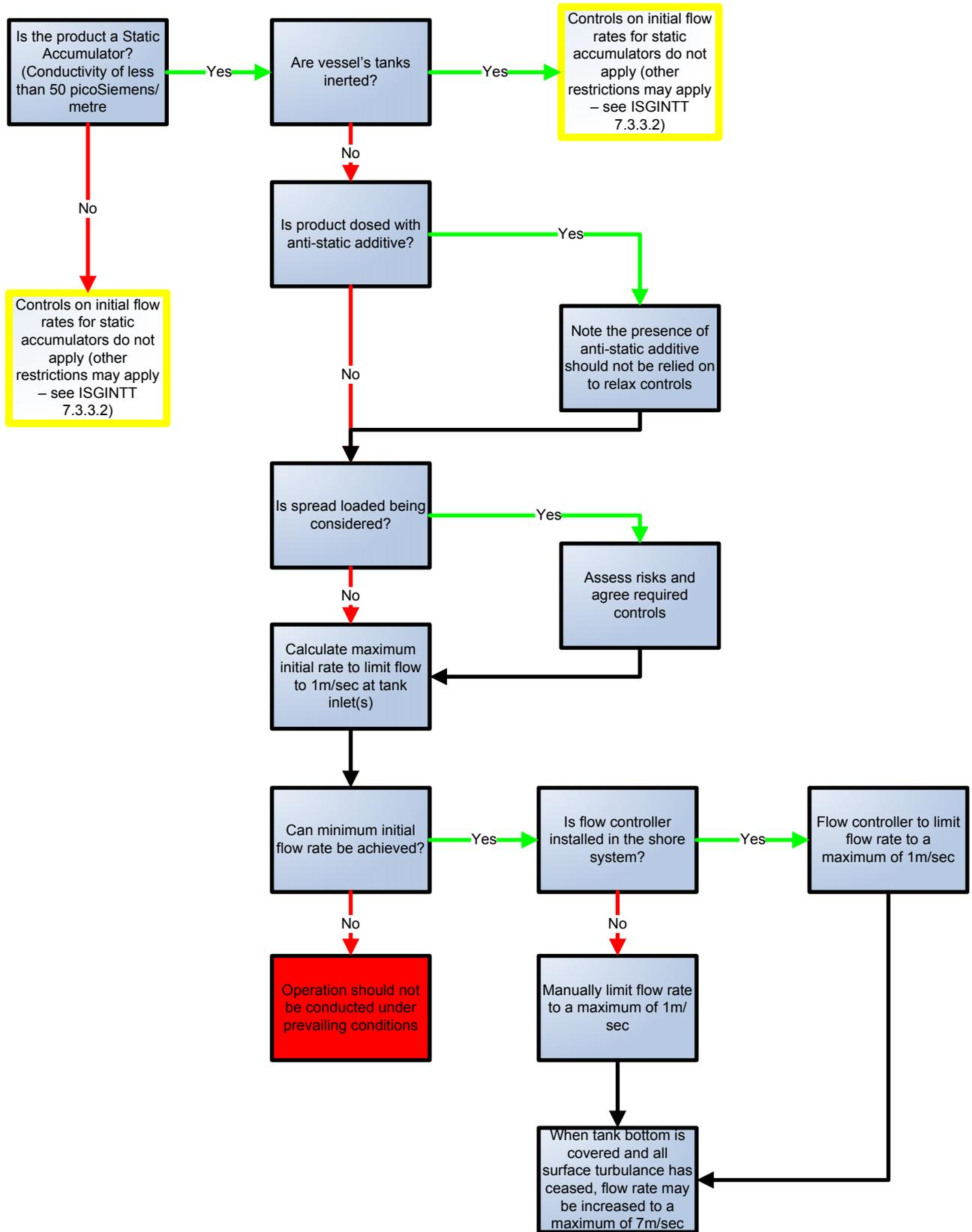
Figure 11.1 - The control hazards associated with the initial loading of static accumulator cargoes
