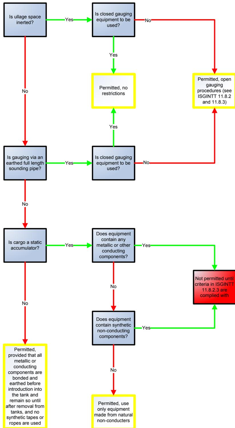
Figure 11.5 - Precautions required when using portable measuring and sampling equipment
