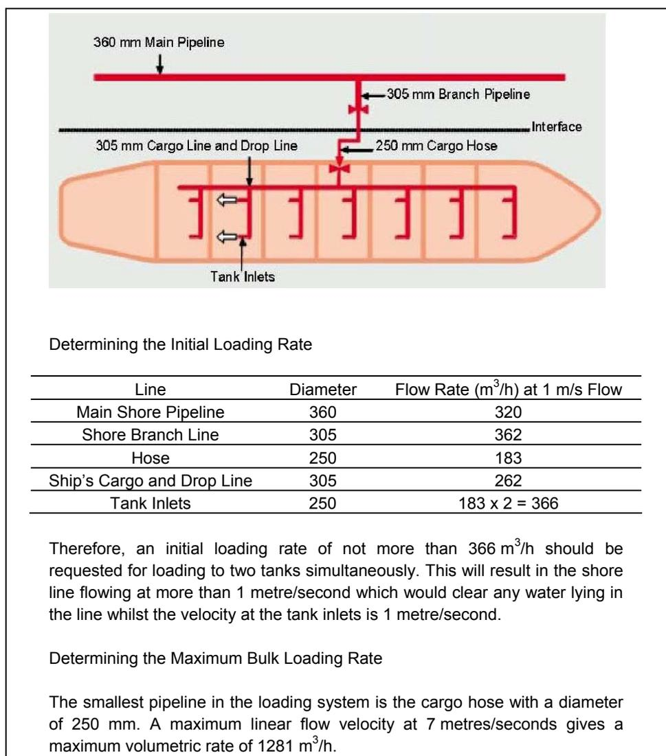
Figure 11.2 – Determining loading rates for static accumulator cargoes
